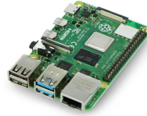
(a) Configuration of the Raspberry Pi 4 with accessories. (b) Single-board view of the Raspberry Pi 4.
